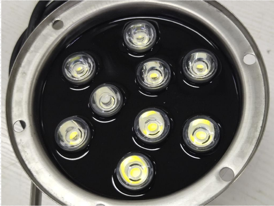
Photo 5: Test result after IP6X and IPX8 test
